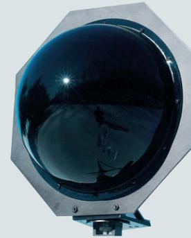
Unlike conventional helical antennas, most of which have a much narrower bandwidth, the A 5000-CP covers the entire UHF range from 450 to 960 MHz. This flexibility makes setting up even the most complex RF transmission systems much easier. The antenna minimizes variations in signal strength and almost completely eliminates multipath problems. The gain of the A 5000-CP over the entire UHF band is superior to that of conventional antennas.
