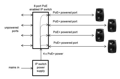
Example of powering the 4430A with a PoE+ enabled IP switch. With this method, the power budget available for all outputs connected to the IP switch must enable each 4430A to run at full PoE+ power. For 4 loudspeakers, the power supply must support  $4 \times PoE+$  power level.
